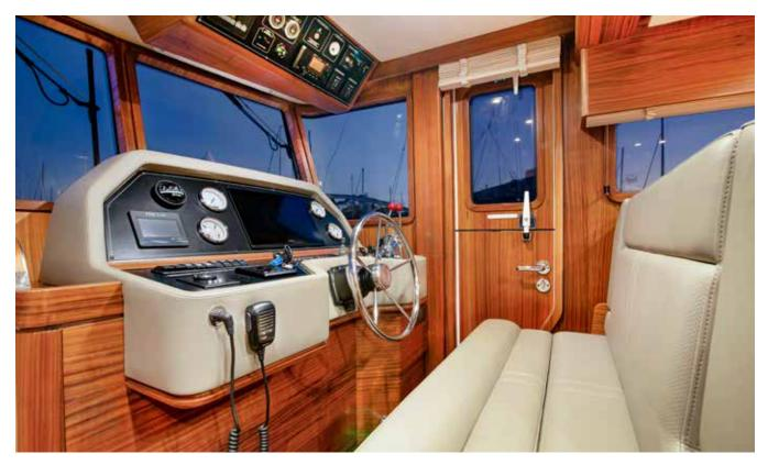
The hooded dash and reverse raked pilothouse windows prevent night reflections, and the dogging Dutch door provides easy deck access as well as a breeze.
